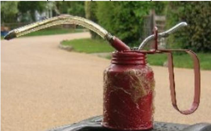
A traditional small engineer's oil can with a moderately long flexible spout and convenient lever actuating a pump mounted in the handle is the ideal piece of equipment for leaning across from the wing and directing a gentle flow of oil into the damper. The pumping action
