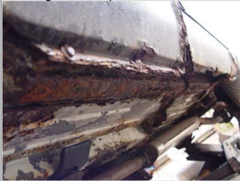
Two examples of rust in the sills and lower rear wing – an area prone to rust
