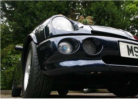
An early Japan spec RV8 with front wheel arch spats and aircon intake grilles> (Photo: Richard Selwyn)
