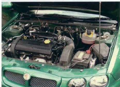
The 1.4K series engine fitted in the ZR produces 105PS.
