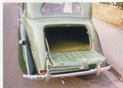
Check the boot lid and spare wheel cupboard for corrosion.
