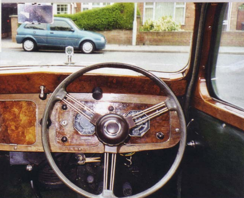
The interior is by far the most expensive to restore. Check it is all there and in good condition. Does opening the windscreen work? Does it leak?
