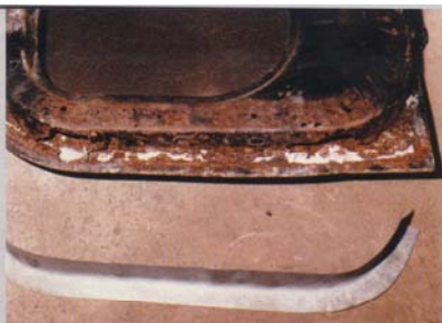
The door bottoms can rot out badly. Photo:- Dennis Doubtfire.
